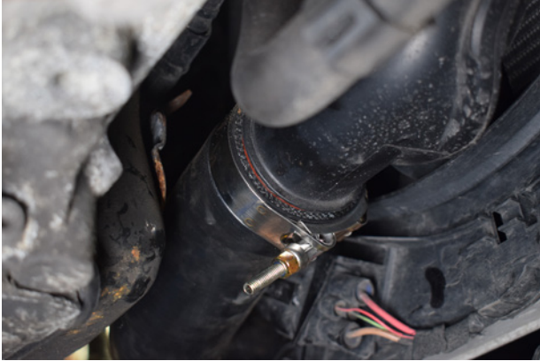
73. Tighten clamps to secure.
