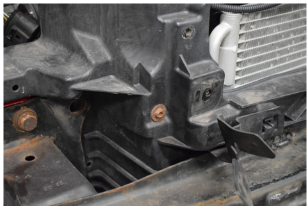
66. Continued to fully secure the plastic slam panel using original hardware.
