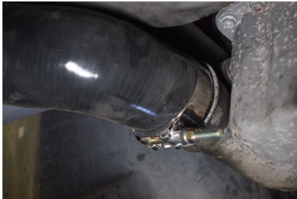
75. Tighten both clamps.
