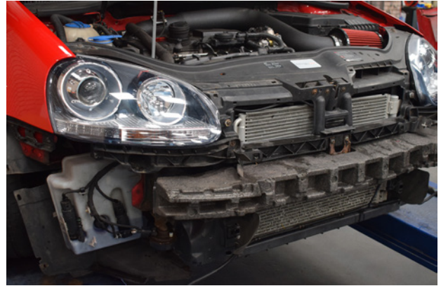
76. With the intercooler installed you can re-fit the front bumper.
