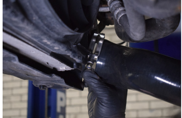
74. repeat this process for the boost pipe on the other side of the car.
