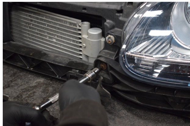
2. Undo the 2x screws to remove the plastic trim below the headlight.
