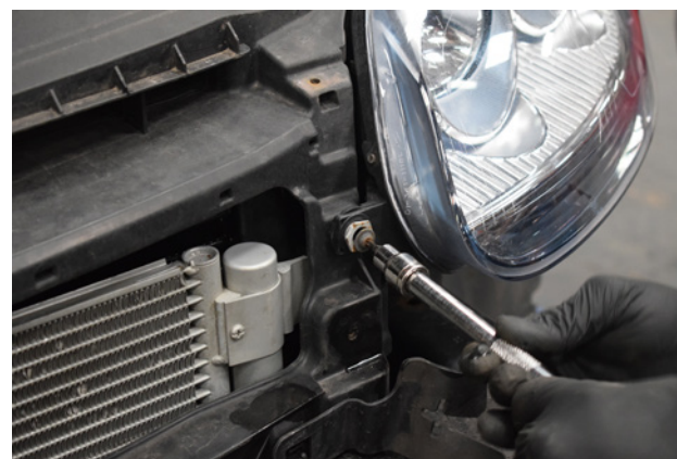
4. You can now undo 3x screws securing the headlight to the car.
