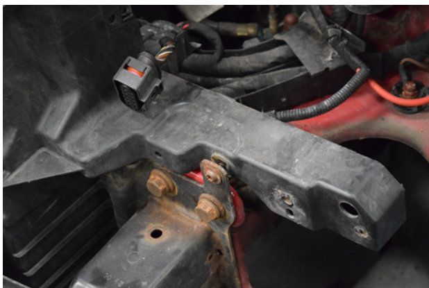
65. Install smaller crash bar mounting screws.
