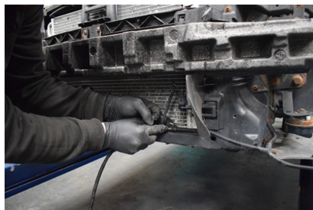
10. Disconnect & un-clip foglight wiring from the front of the car.
